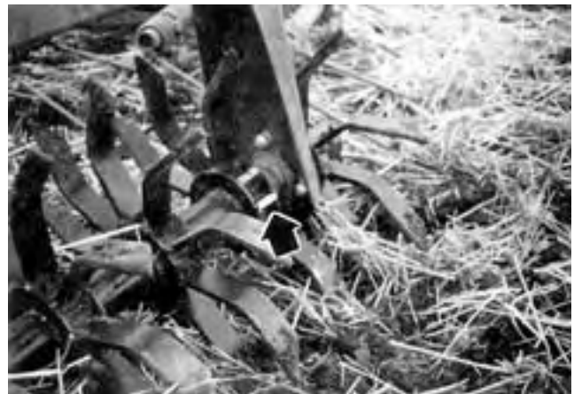
FIGURE 8. Broken Teeth on the Original Weeders.
