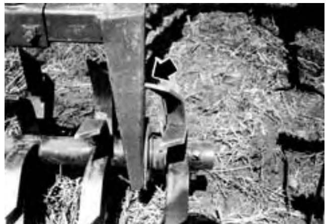
FIGURE 9. Bent Teeth Stopping Rotation.
