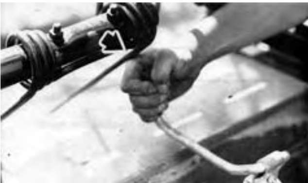
FIGURE 8. Interference Between Jack Handle and Harrow Tine Bar.
