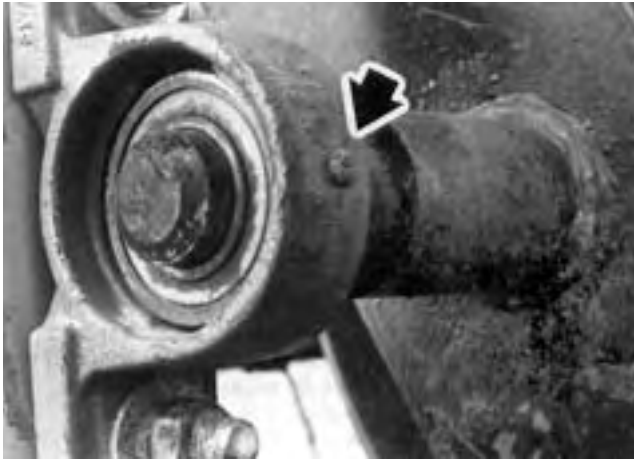
FIGURE 9. Damaged Packer Grease Fitting.
