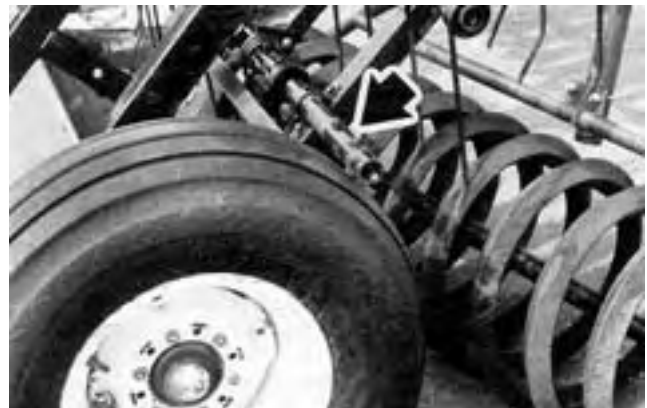
FIGURE 7. Harrow Tine Removed to Prevent Tire Interference with Wing Wheel.
