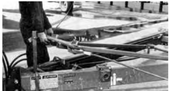
FIGURE 5. Operator Lifting the Wing Cable Pivot Arm for Transport Position.
