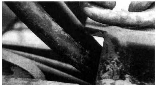
Figure 13. Damaged Depth and Wing Hydraulic Lines.
