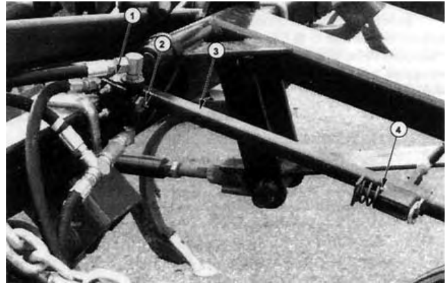
Figure 10. Depth Stop Adjustment System. (1) Depth Stop, (2) Shut-off Needle, (3) Depth Stop Rod and (4) Depth Stop Adjustor Assembly.
