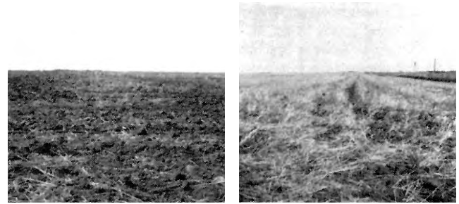
FIGURE 9. Trash Burial of the Lely S-8-6 (left) Compared to that of a Blade Cultivator (right).
