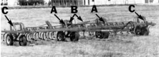
FIGURE 1. Hesston 2210: (A) Master Cylinders, (B) Wing Lift Cylinder, (C) Slave Cylinders.
