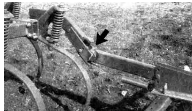
FIGURE 10. Harrow Support Arm Failure.
