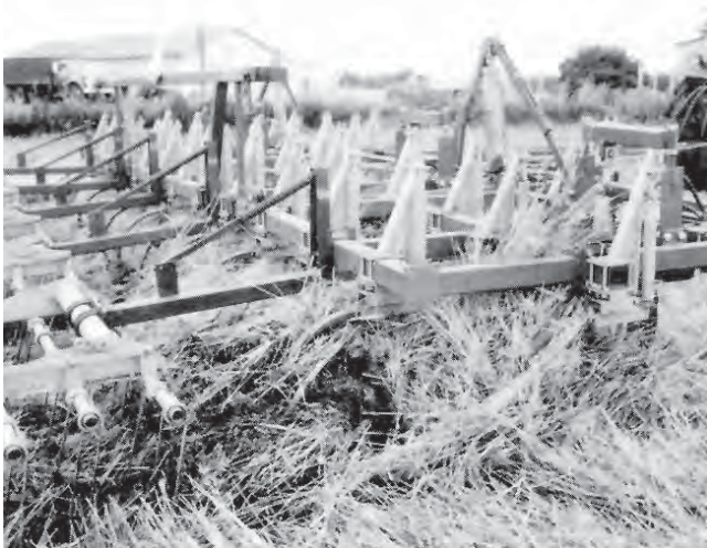
FIGURE 5. Plugging Beside the Wing Wheel in Long Wheat Stubble.
