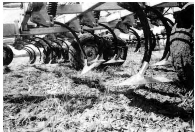
FIGURE 11. Shank Bent After Contacting the Frame.
