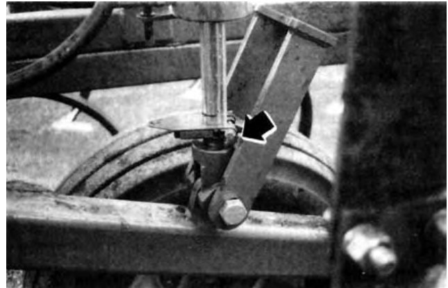
FIGURE 10. Interference Between Depth Stop and Transport Locks.
