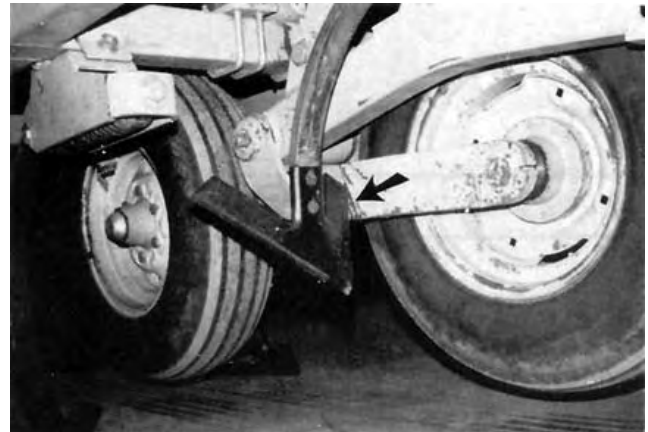
FIGURE 12. Reduced Shank Clearance at Wheel Locations.
