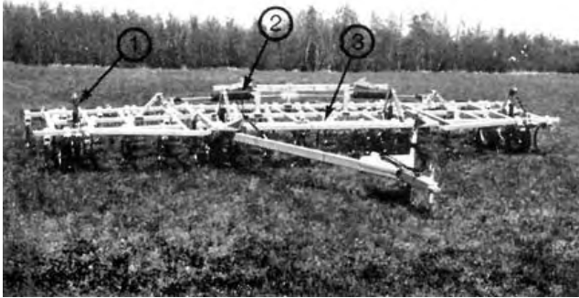
FIGURE 1. Degelman 3000 (1) Depth Control Cylinders, (2) Wing Lift Cylinders, (3) Hydraulic Flow Divider.
