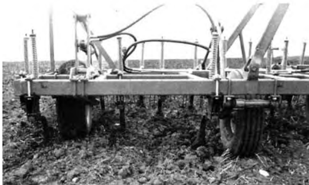
FIGURE 5. Secondary Wing Wheel Positions Before Modifications.
