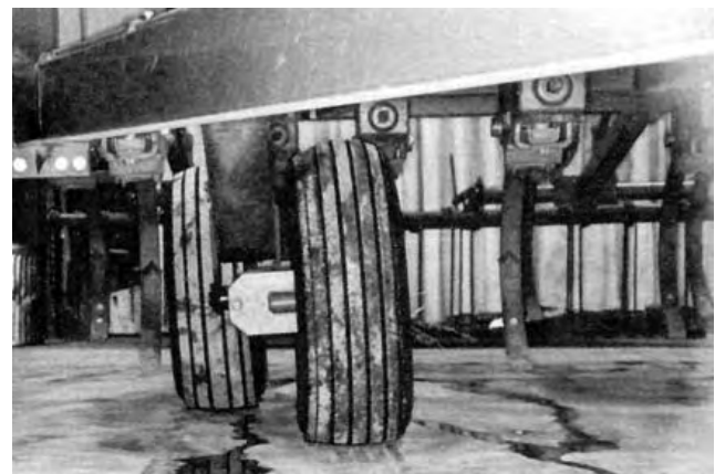
FIGURE 11. Centre Section Wheel Support Deflection in Transport Position.
