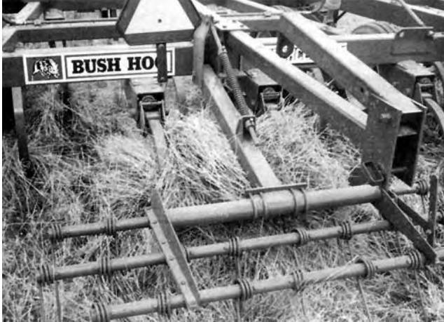
FIGURE 5. Plugging Between the Centre Shanks and Finishing Harrows.
