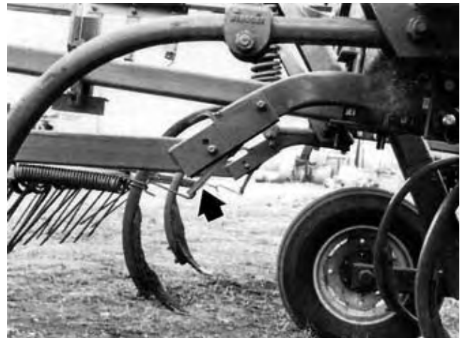
FIGURE 12. Bent Harrow Spring Mount.
