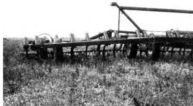
FIGURE 5. Excessive Wing End Penetration in Heavy Primary Tillage.
