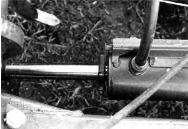
FIGURE 10. Hydraulic Depth Control Stop and Transport Lock.
