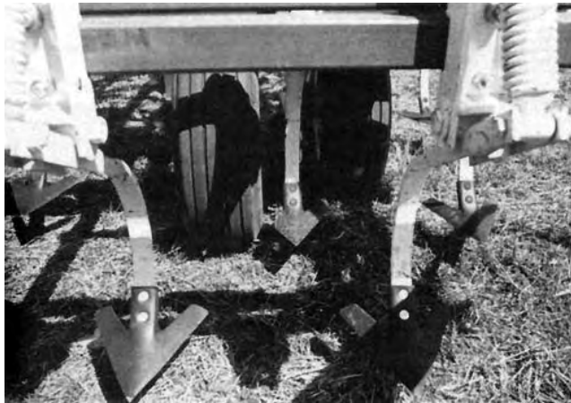
FIGURE 10. Trimmed Sweeps Adjacent to Centre Section Wheels. FIGURE 11. Average Draft Requirements for Field Cultivators at 8 km/h.
