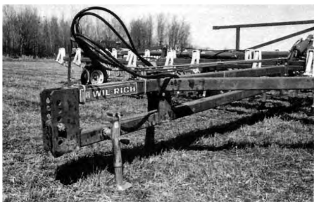
FIGURE 8. Hitch Link in Vertical Position.
