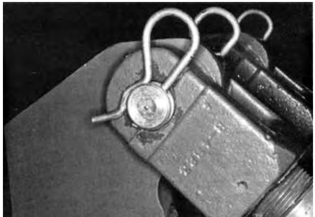
FIGURE 13. Damaged Retainer Clips on Cylinder Yokes.
