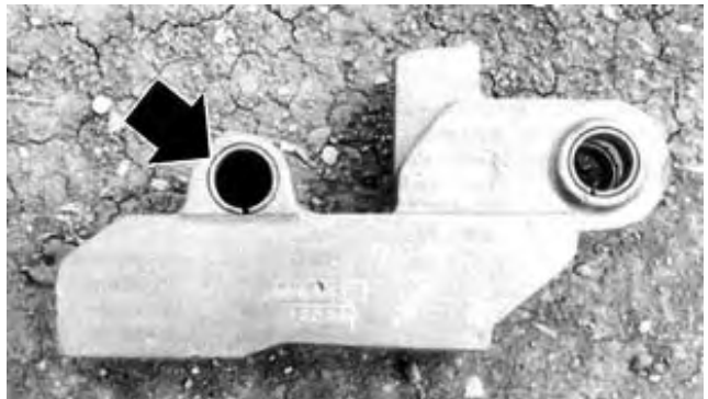
FIGURE 17. Re-designed Release Shoe Showing Properly Drilled and Bushed Main Pivot.
