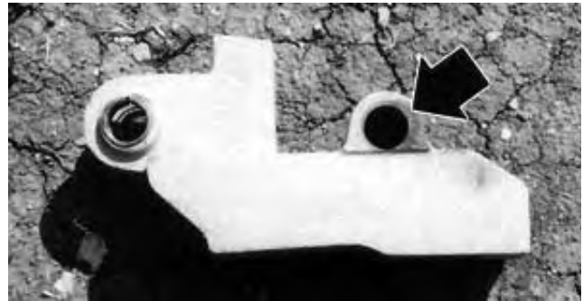
FIGURE 16. Original Shank Trip Release Shoe Showing Improperly Drilled Main Pivot.
