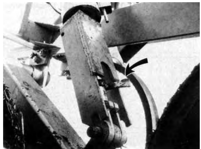
FIGURE 13. Interference of Safety Lock with Depth Control Stop.
