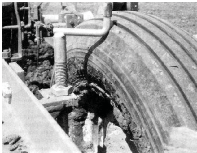
FIGURE 8. Interference of Depth Stop Crank with Depth Control Wheel.
