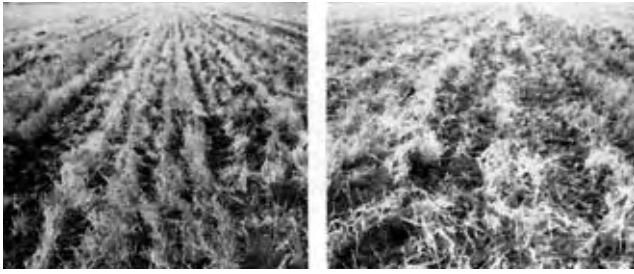
FIGURE 5. Trash Burial with 47 Degree Sweeps at 75 mm Depth at 6 km/h (Left) and 10 km/h (Right).
