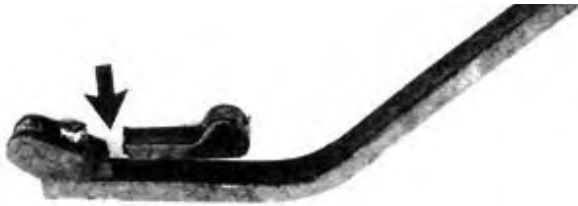
FIGURE 12. Broken Shank Attaching Casting.
