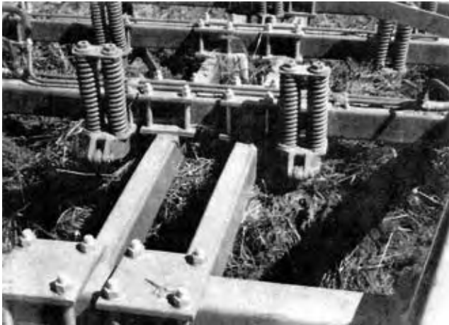
FIGURE 5. Plugging at Two Centre Shanks.
