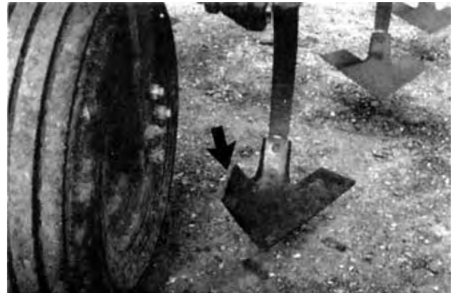
FIGURE 10. Sweep Wing Cut-off to Prevent Tire Damage.
