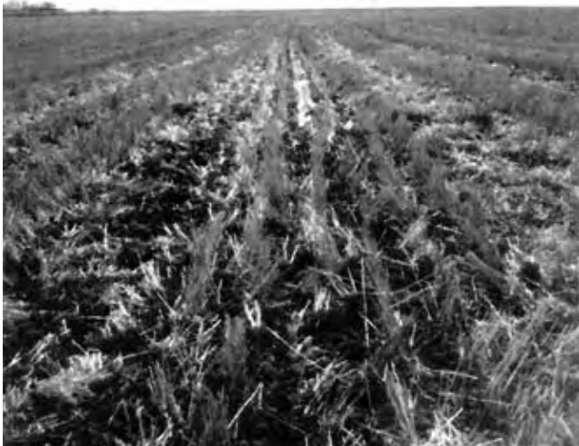
FIGURE 5. Trash Burial with 50 Degree Sweeps at 6 km/h and 75 mm Depth.
