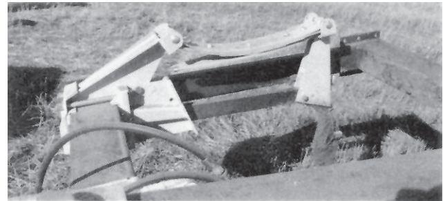
FIGURE 13. Over Centred Leaf Spring.
