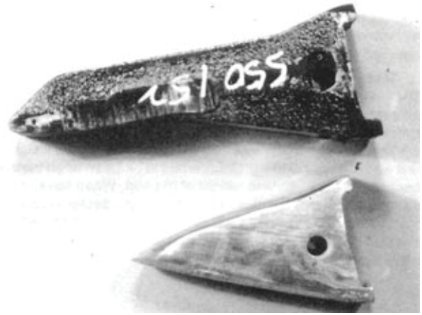
FIGURE 9. Point Wear: Top - New Point, Bottom - Worn Point.
