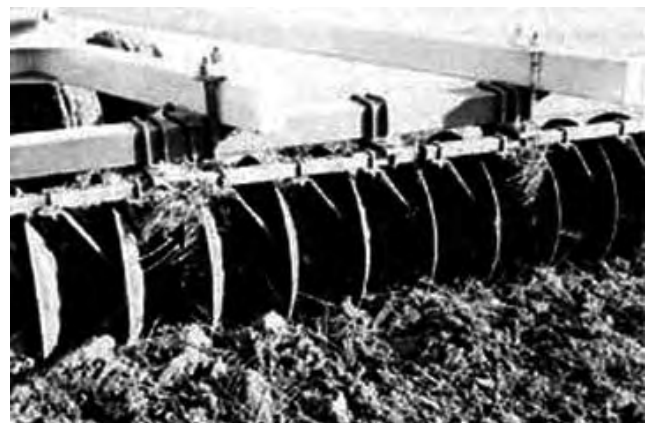
FIGURE 2. Trash Build-up Between Scrapers and Gang Bearing Hangers.
