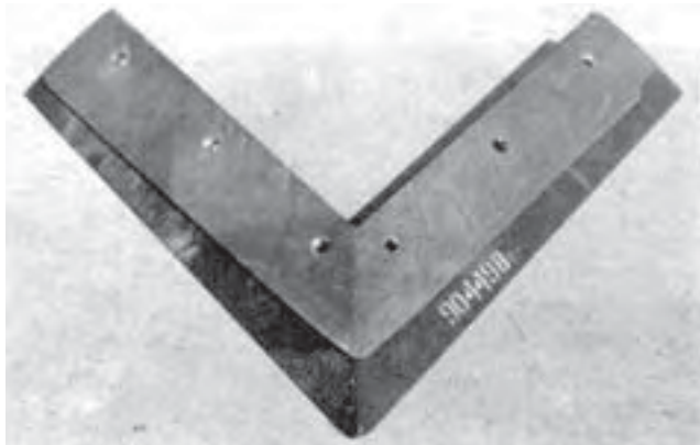
FIGURE 16. Typical Wear on Plain Sweep During the Test.
