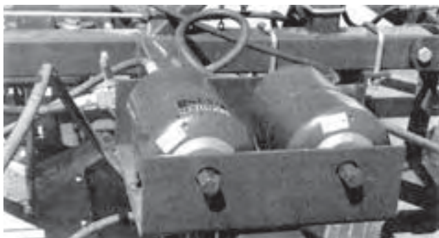
FIGURE 2. Nitrogen Charged Accumulators.
