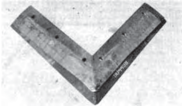
FIGURE 15. Typical Wear on the Top Hardfaced Sweep During the Test.
