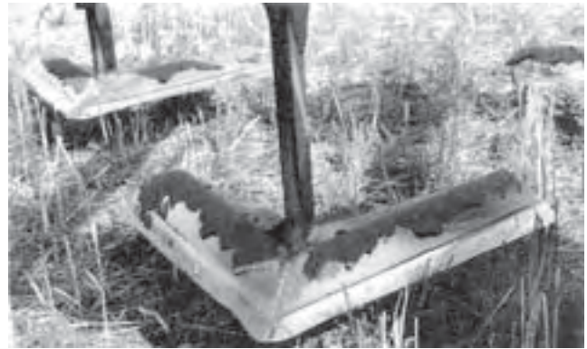
FIGURE 8. Poor scouring of sweeps.
