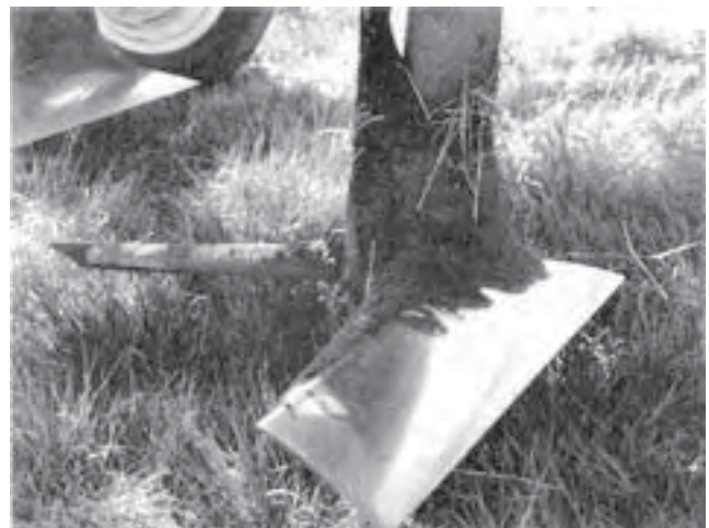
FIGURE 10. Soil Built Up Around Standard and Fertilizer Distribution Tube.
