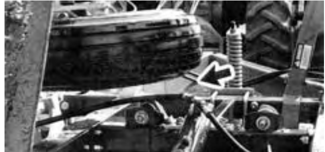
FIGURE 18. Small Clearance Between Tire and Hydraulic Tee at Start of Test.
