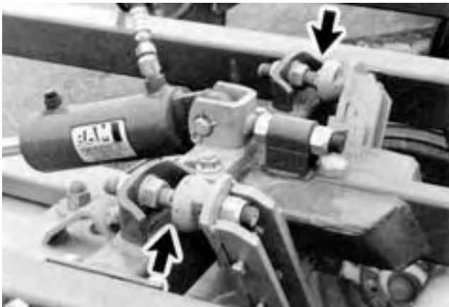
FIGURE 12. Adjustable Round Ended Socket Pins.
