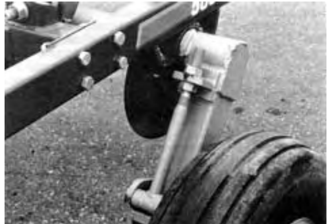
FIGURE 14. Adjustable Axle Tee-Bolts.
