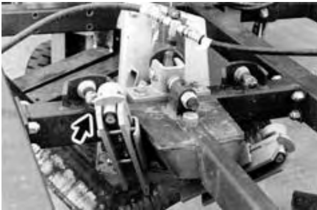
FIGURE 7. Binding Linkage with Side Tripping.
