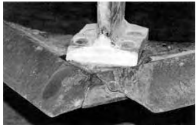
FIGURE 10. Nose Broken Off Blade.
