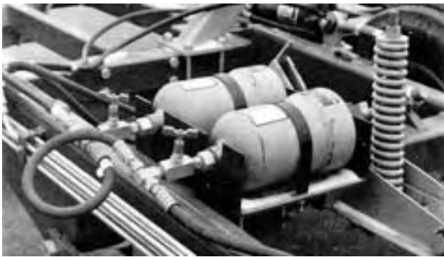
FIGURE 2. Nitrogen Charged Accumulators.
