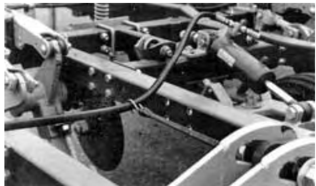
FIGURE 19. Tarp Strap Used to Keep Hydraulic Hose from Rubbing on Tire.
