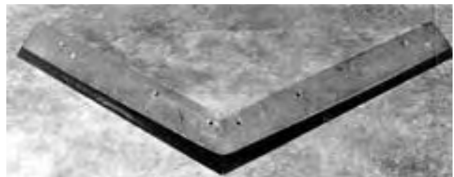
FIGURE 20. Wear on Typical Blade at End of Test.
