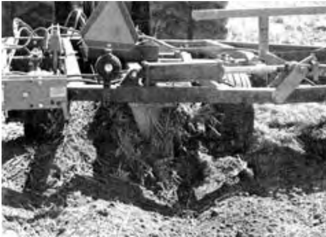
FIGURE 5. Plugging at the Centre Shank.
