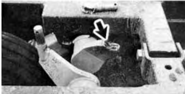
FIGURE 10. Turnbuckle Pin Failure.
