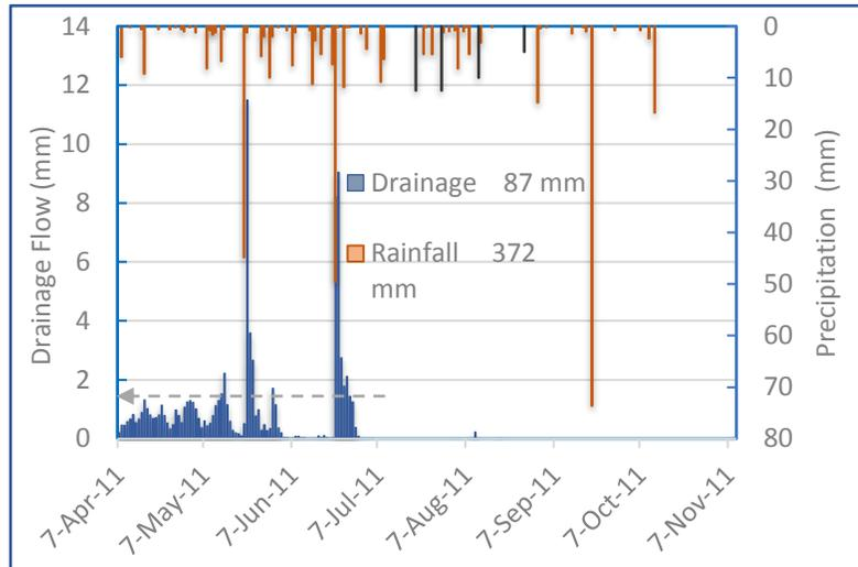
**Figure 5. Drainage flow vs. precipitation for Hespler Farms research plot (Cordeiro, 2013); arrow represents 1.6 mm/day maximum treatment rate.**
