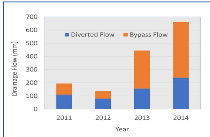
Figure 4. Flow diverted to riparian zone (buffer strip vs flow bypassing riparian zone at Bear Creek (Iowa) (Jaynes et al.; ADMC website).
