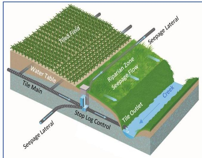
Figure 2. Plan view of saturated buffer, including stop log control structure, seepage lateral and riparian zone parallel to the outlet waterway (source: modified from TransformingDrainage.Org).
