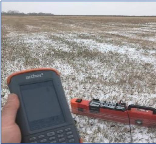
**Figure 3. Field investigation using EM38 mapping for soil texture variability and salinity.**
