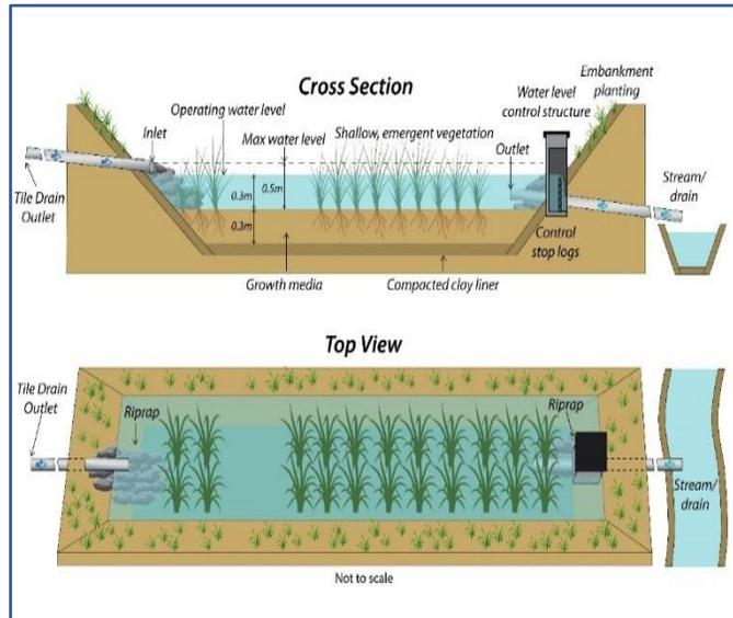
Figure 2. Conceptual diagram of components and layout of a constructed wetland.
