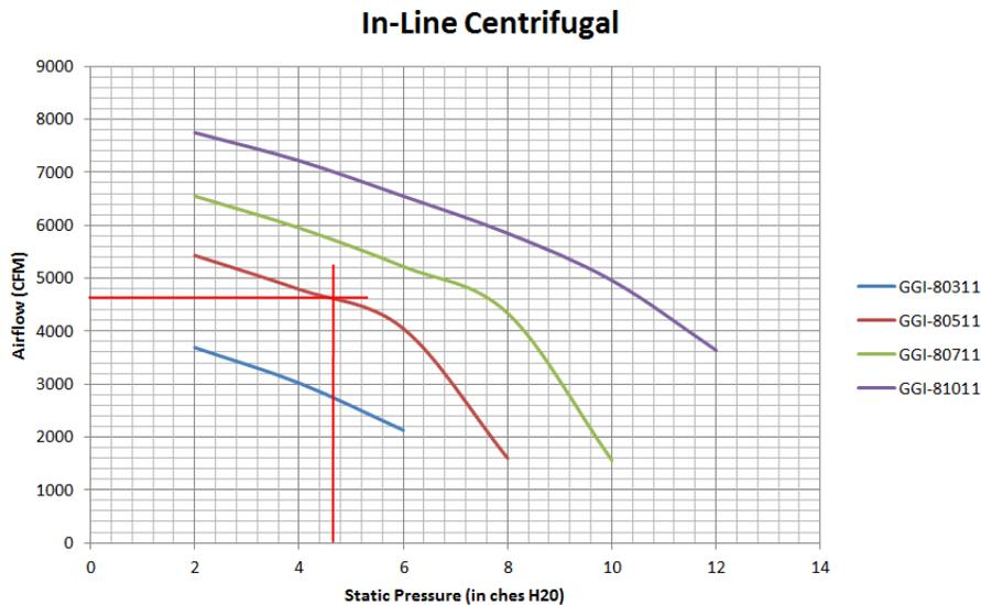
Figure 1. Example of airflow performance data for Grain Guard in-line centrifugal fans (same information shown in Table 1 shown in a different way).
