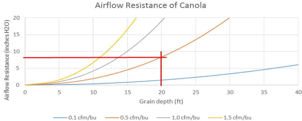
Figure 2. Estimated airflow resistance (static pressure) for canola.
