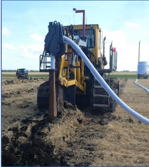
**Figure 1. Installation of tile drainage on an agricultural field.**
