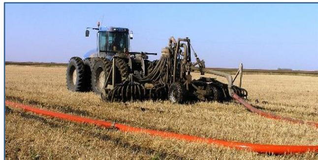
**Figure 5. Example of manure injection technology.**
