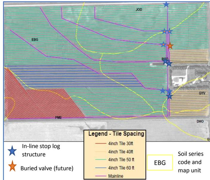
Figure 5. Typical controlled drainage design in Manitoba.
