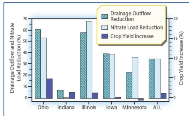
**Figure 3. Drainage outflow and nitrate load reduction and crop yield increase resulting from controlled drainage vs. conventional drainage systems (Christianson et al., 2016).**
