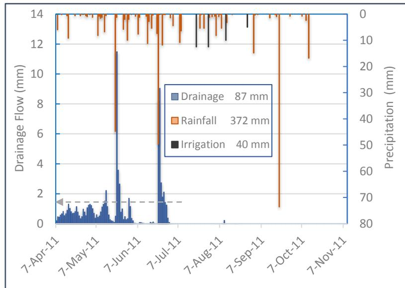
**Figure 4. Typical tile drainage flow from a fine sandy loam on the Hespler Farms research plot (Cordeiro, 2013); arrow represents bioreactor sized for 25% of a 6.35 mm/day (0.25 in/day) drainage coefficient.**
