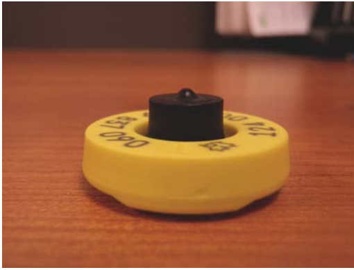
Figure 1 Radio Frequency Identification (RFID) tags are an important part of tracking individual cows from birth to slaughter, but some producers report poor retention after installation.
