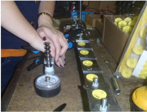
Figure 2. The insertion force required to apply the RFID tags was tested during the PAMI research team's test procedures.
