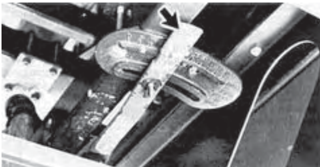
FIGURE 14. Seeding Rate Selection Lever.
