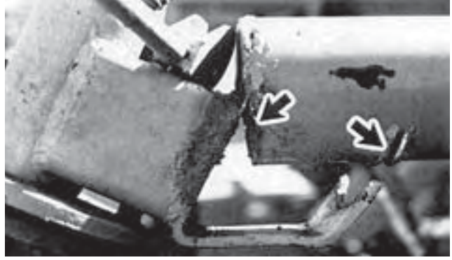
FIGURE 16. Transport Wheel Mount Weld Failure.
