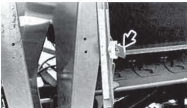
FIGURE 15. Fertilizer Rate Selection Lever.
