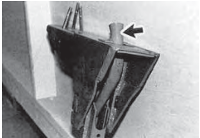
FIGURE 17. Coiled Steel Deliver Tube Adapter: (Upper) Front Row Adapter, (Lower) Middle and Rear Row Adapter.
