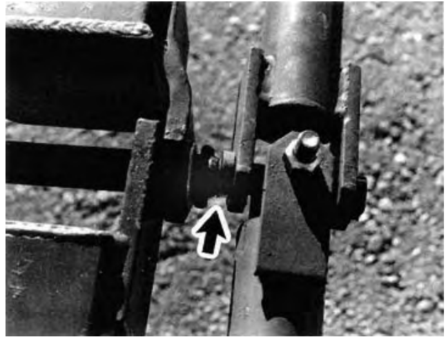
FIGURE 12. Spray Boom Universal Joint and Boom Pivot Pin.
