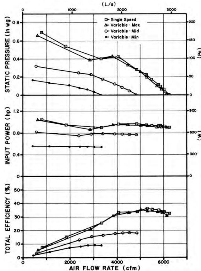
FIGURE 3. Ziehl-Abegg 562-6 Fan Performance Curves in the Single Speed Mode and at Three Speed Settings in the Variable Speed Mode.
