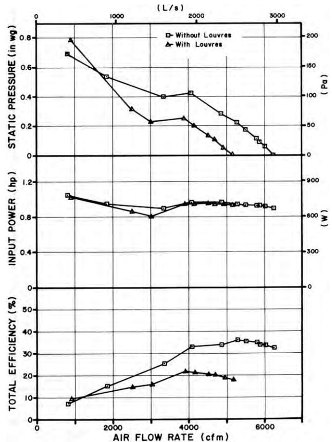
FIGURE 5. Effect of Louvres on Fan Performance.
