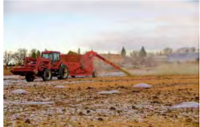
Figure 3. Distribution of dry hay directly onto ground at 540 rpm PTO speed.
