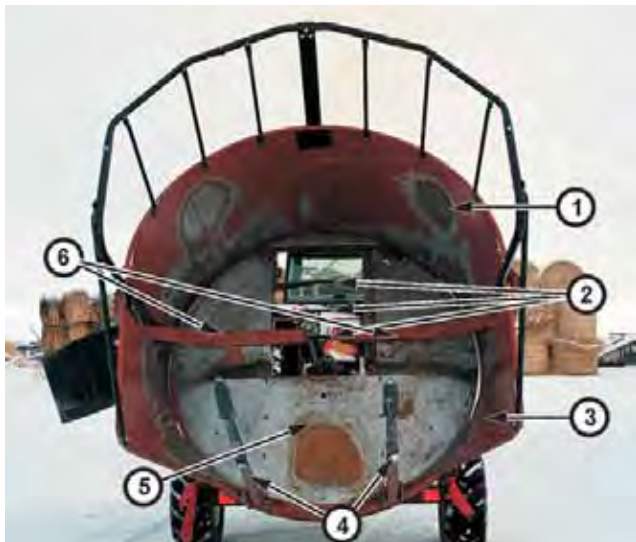
Figure 2a. (1) Tub/Chamber, (2) 3 Grid bar rotor guards, (3) Chamber hydraulically tilted 90°, (4) Bale lifting forks, (5) Tub floor, (6) Bale driver arms.
