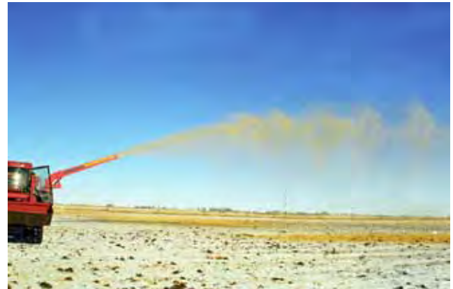
Figure 4. Highline Top Gun distributing dry straw at the maximum height.
