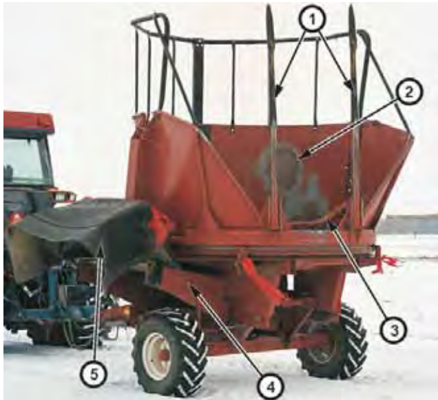
Figure 1. (1) Bale forks, (2) Tub/Chamber, (3) Bale driver arms, (4) Distribution chamber, (5) Upper side deflector.
