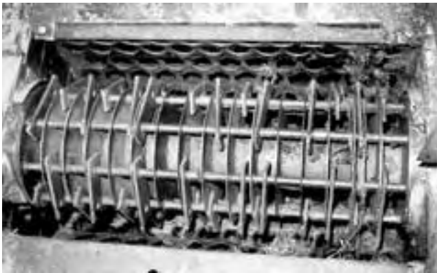
FIGURE 3. Hammer Mill and Screen.
