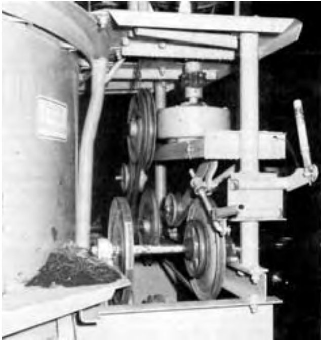
FIGURE 2. Sheaves for Tub Speed Control.
