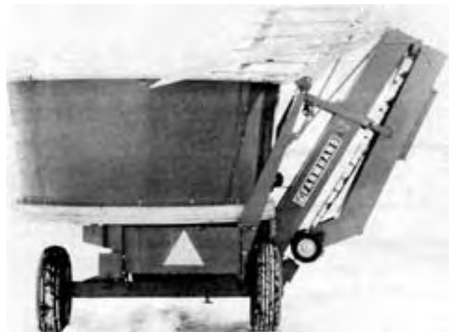
FIGURE 6. Elevating Conveyor in Transport Position.
