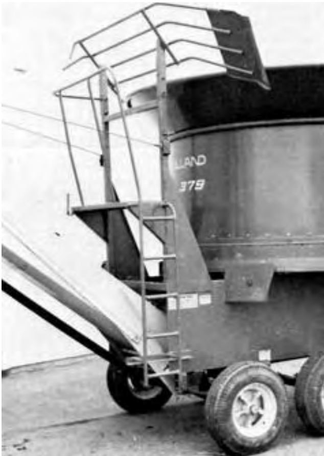
FIGURE 9. Guide Rack and Winch Cables.
