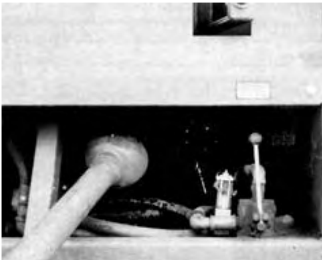
FIGURE 10. Tub Speed Controls.
