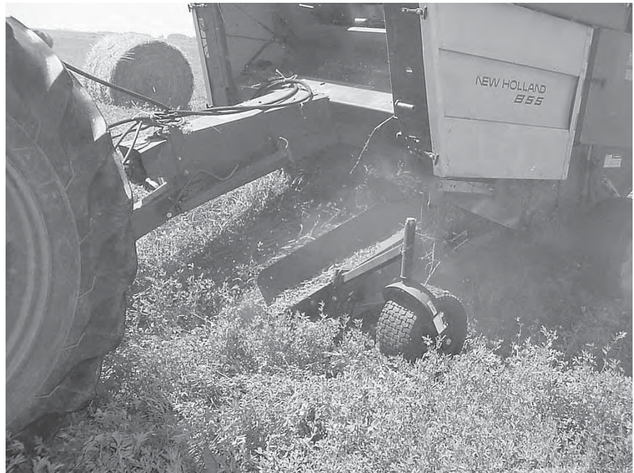
Draper header on a New Holland 855 round baler.
