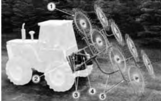
FIGURE 1. Vicon H1240 Trapeze V-Rake: (1) Finger Wheels, (2) Main Frame, (3) Width Adjustment Brackets, (4) Adjustable Tension Springs, (5) Fingerwheel Frames.
