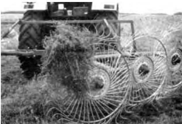
FIGURE 4. Windblown Crop Falling Behind Finger Wheels.
