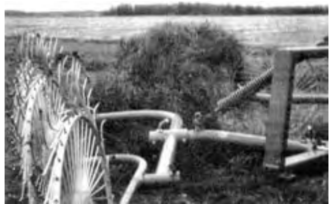
FIGURE 5. Crop Bailing Up and Rolling in Front of the Finger Wheels.
