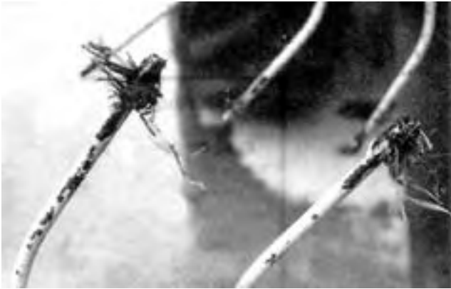
FIGURE 2. Soil Sticking to Tips of Fingerwheel Tynes.
