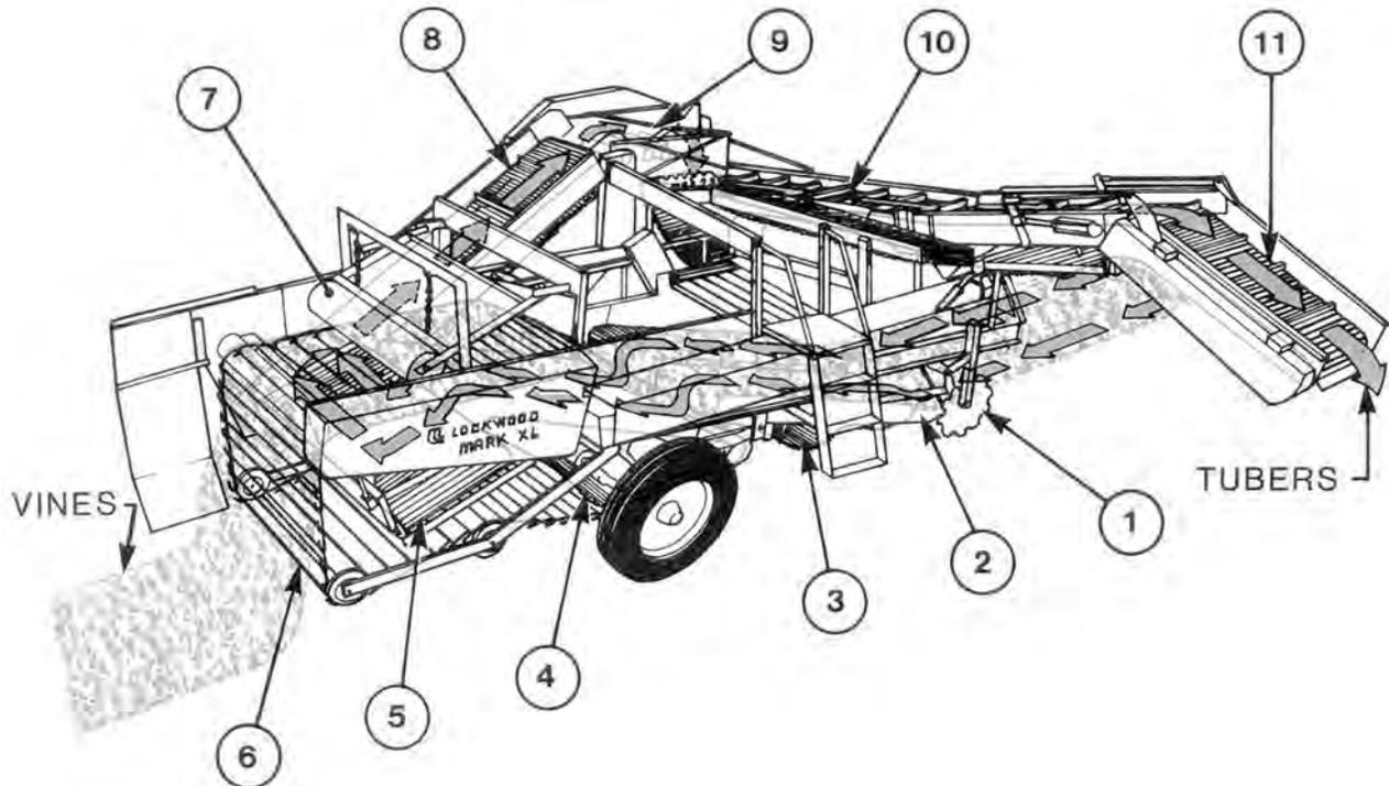
FIGURE 1. Lockwood Mark XL Potato Harvester. (1) Coulters, (2) Spade, (3) Primary digger chain, (4) Secondary digger chain, (5) Cross conveyor, (6) Deviner, (7) Stripper roller, (8) Elevating conveyor, (9) Star clod table, (10) Sorting table, (11) Delivery boom.
