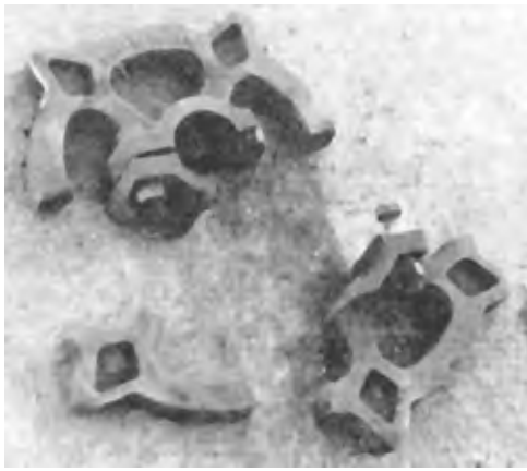
FIGURE 5. Deviner Chain Cast Iron Drive Sprocket.
