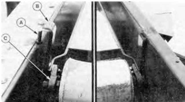
FIGURE 6. Failure of Support Strap on Stripper Roller: (A) Adjustment Bolt, (B) Support Strap, (C) Hanger Bearing.
