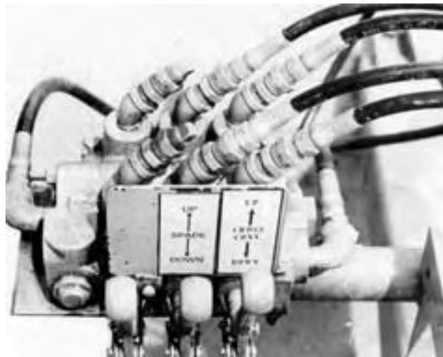
FIGURE 2. Hydraulic Control Valve Assembly.
