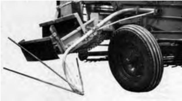
FIGURE 3. Optional Vine Divider in Working Position.
