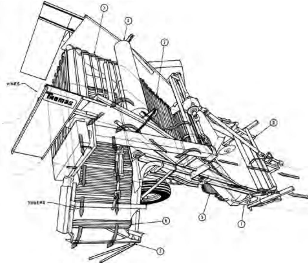
**FIGURE 1.** Thomas 660 Potato Windrower: (1) Coulters, (2) Vine Lifter, (3) Deviner Chain, (4) Stripper Roller, (5) Primary Digger Chain, (6) Cross Conveyer Boom, (7) Secondary Digger Chain, (8) Coulters Lift Arm.
