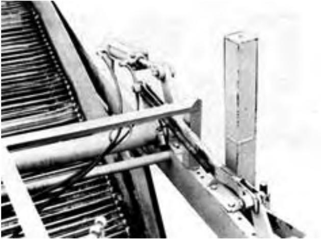
FIGURE 5. Coulters Activating Arm.
