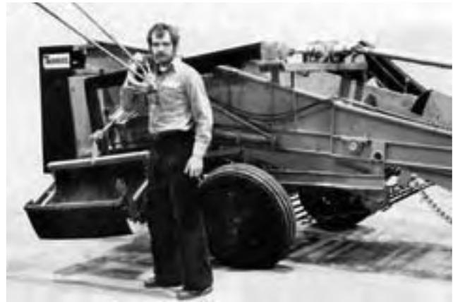
FIGURE 4. Potential Eye Hazard Caused by Vine Divider
