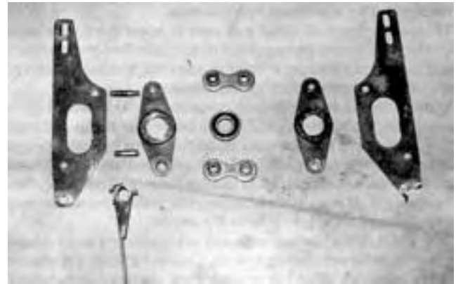
FIGURE 4. Failed Knife Drive Mechanism.
